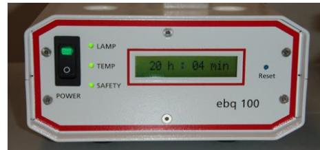
The lamp is ready to use immediately the arc strikes but takes a few minutes to stabilise fully and warm up to maximum intensity.
